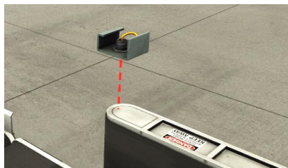
Figure III. 89 Feedback Sensors: Capacitive Sensors on Pivot Arms
